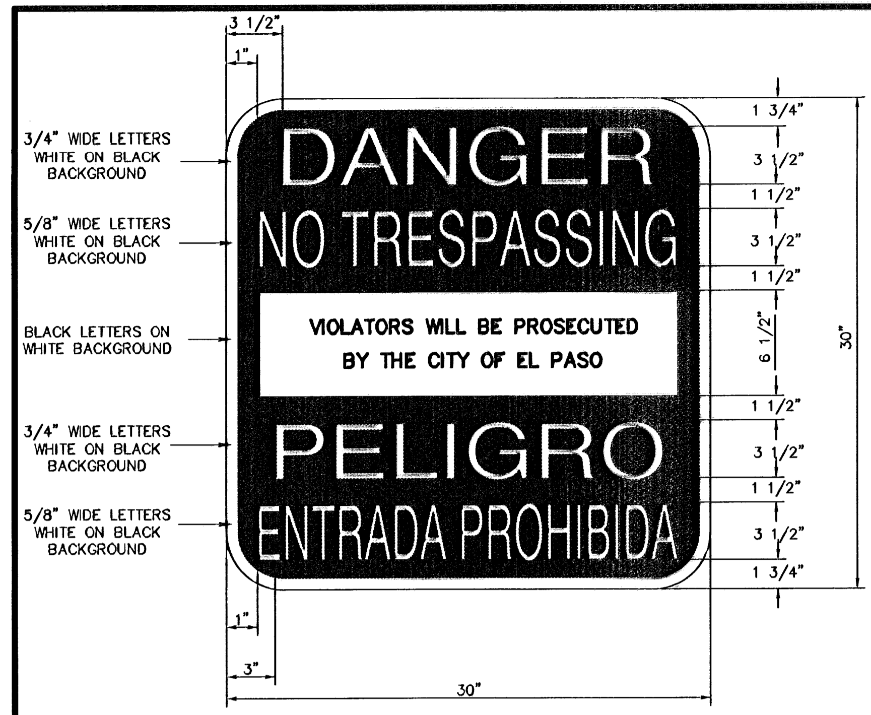
1 NO TRESPASSING WARNING SIGN SCALE: NTS
