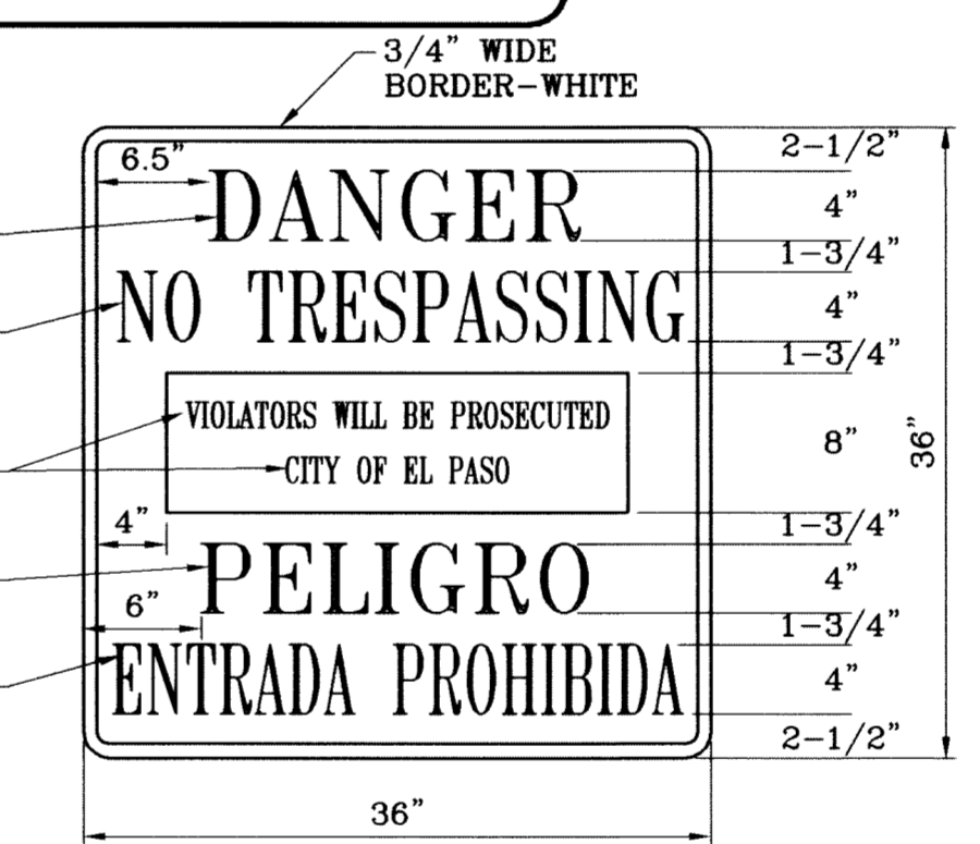
WARNING SIGN DETAIL SCALE: 1"=1'
